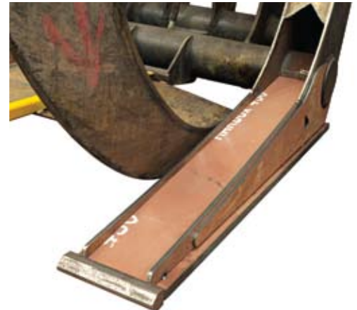
New Alloy Steel Fork Plates Are Fabricated And Welded To Grab
