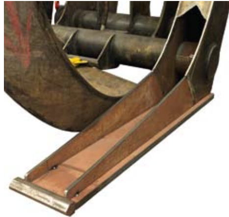
New Alloy Steel Fork Plates Are Fabricated And Welded To Grab
