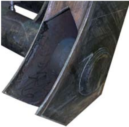
Damaged Leg Plates Are Cut Away
