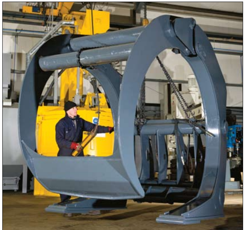
New Alloy Steel Fork Plates Are Fabricated And Welded To Grab
