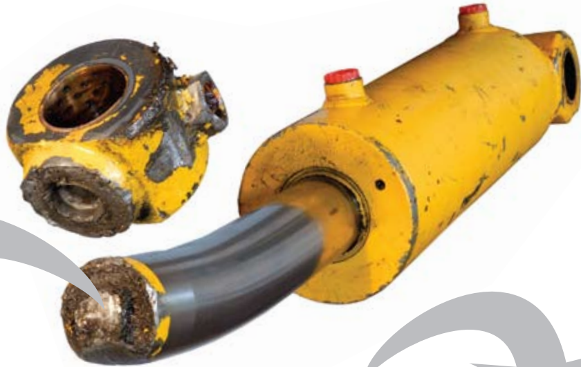
Broken Gland Cap & Bent Shaft
