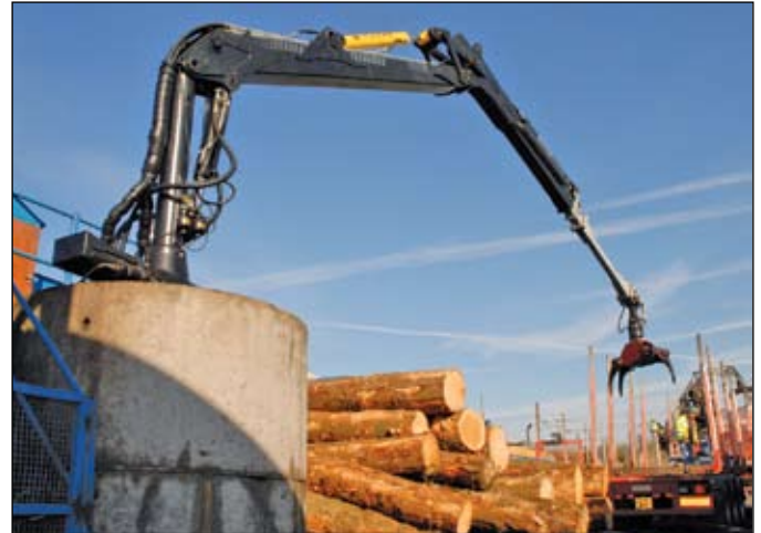
Static Mounted Crane on Concrete Base
