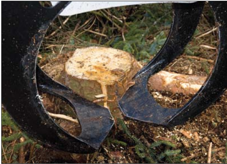
New Tapered X Jaw Profile Allows Easier Movement Around Forest Floor Obstacles
