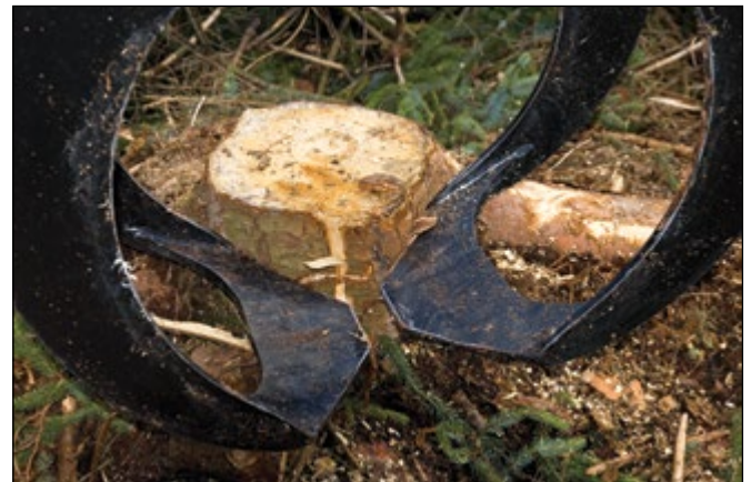
New Tapered X Jaw Profile Allows Easier Movement Around Forest Floor Obstacles
